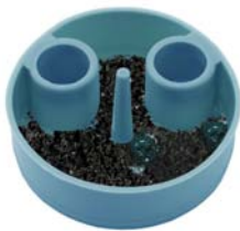
FIGURE 3 - Sludge, bacteria and debris in operator trap.
